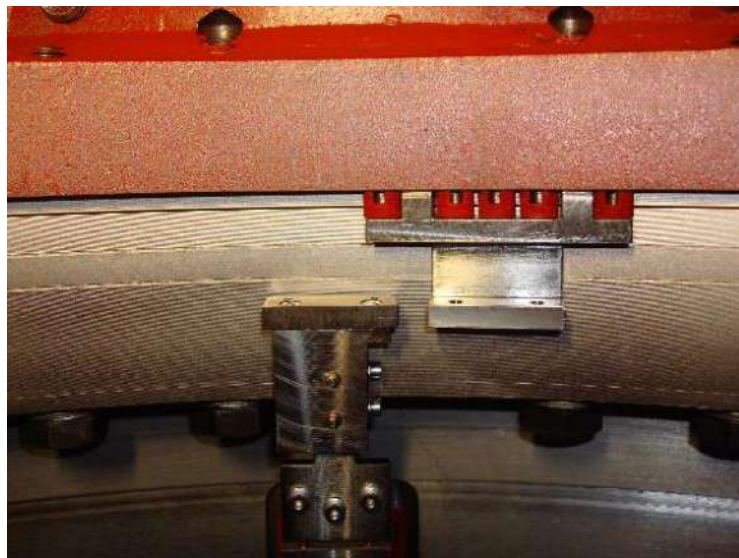
Figure 26 Scanning head dummy before installation on scanning head support
