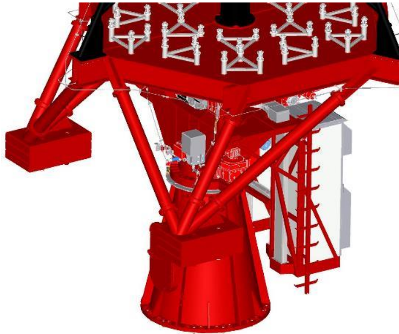
Figure 3-6 Counterweights installed
