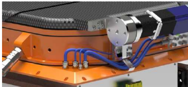
Figure 86: Motor cable routing through Transition Plate via grommets.
