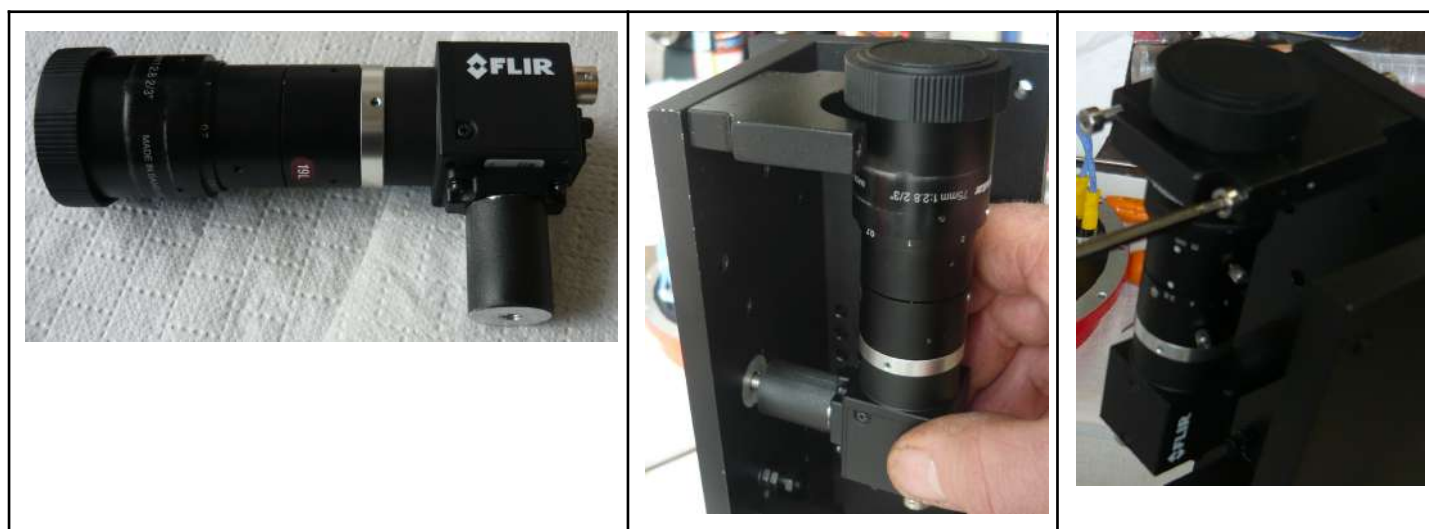
Figure 18. A picture of the PMC Camera and Lens assembled together with the metal cylinder used to anchor the camera to the main mechanical frame (left). The PMC/Lens while being mounted on the internal mechanical frame (centre and right).
