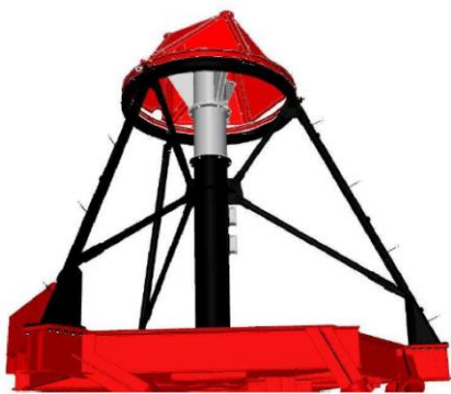
Figure 4-4: Secondary mirror structure in place (courtesy of EIE Group SRL)
