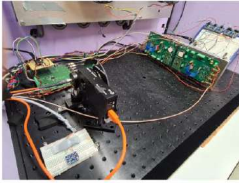
Figure 74: Left: SiPM, preamplifier and shaper tests at the University of Leicester. Right: Resulting performance, showing average pulse shapes from 2 p.e. to ~1800 p.e. Beyond ~500 p.e., once saturation starts to occur, charge-reconstruction will make use of the increasing pulse width.
