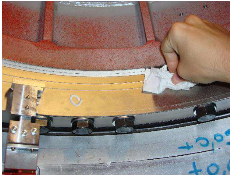
Figure 27 Encoder tape slot cleaning before glueing
