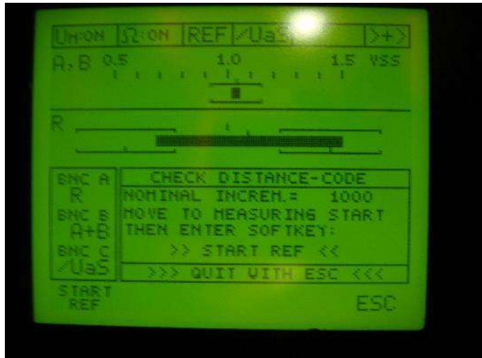
Figure 29 Encoder reading head during calibration and screen of the quality signal
