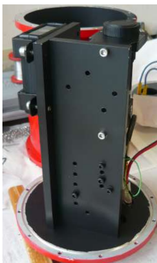
Figure 3. SQM/PMC assembly (top). Main mechanical frame (bottom).
