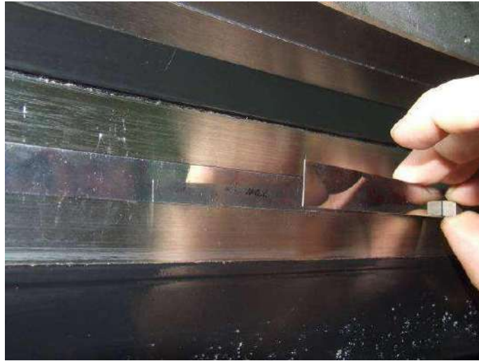
Figure 25 Encoder blank tape installation
