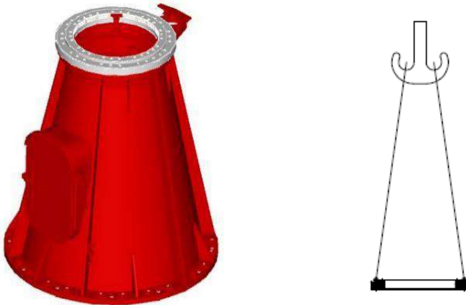
Figure 3 AZ bearing installed and lifting method
