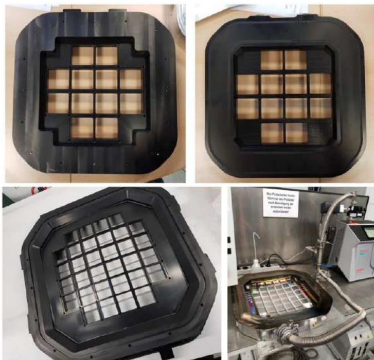
Figure 69: Top: FPP test piece (front: left & back: right). Bottom: Full FPP (left), and under leak test (right).
