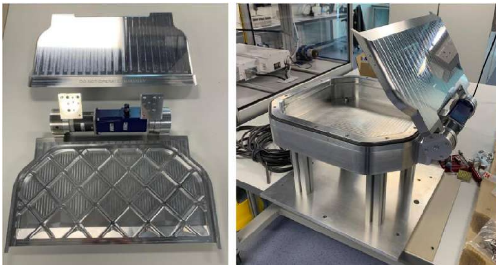
Figure 71: Left: First set of doors on the bench. Right: Small door half with motor, mounted to dummy FPP & Window Frame.
