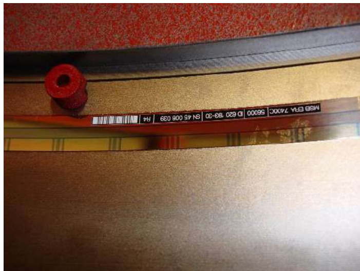
Figure 28 Encoder tape positioned and glued on its slot
