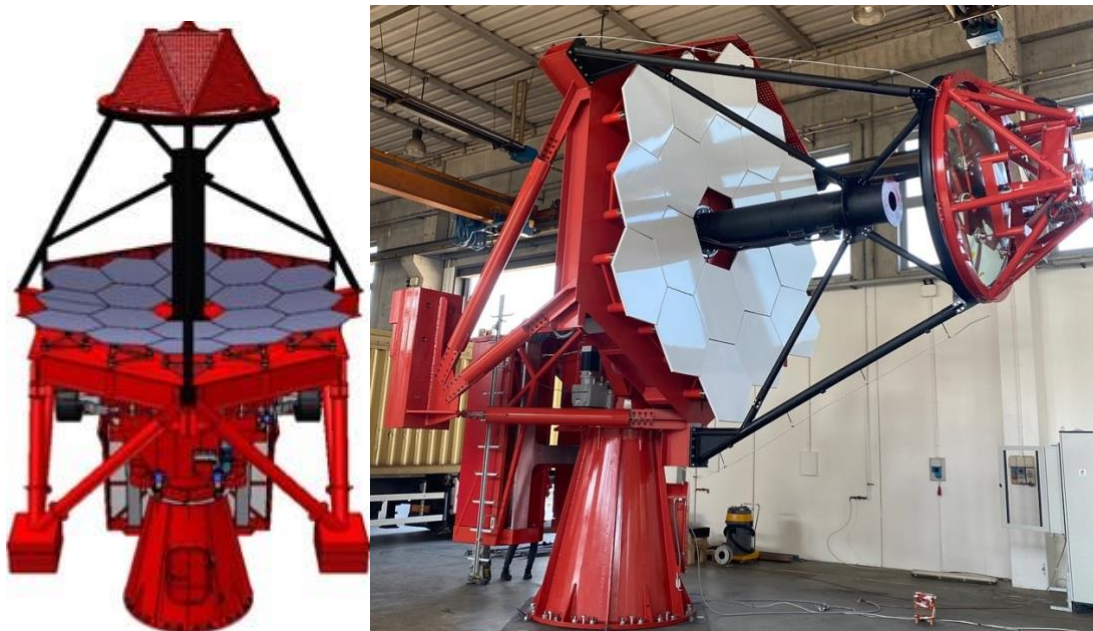
Figure 3-2: left: a 3-D model of the SST telescope structure; right: the first ASTRI Mini-Array telescope fully assembled in a warehouse in Italy before being shipped to the Tenerife Canary Island. This is also the baseline of the SST telescopes, currently under study for further possible improvements.
