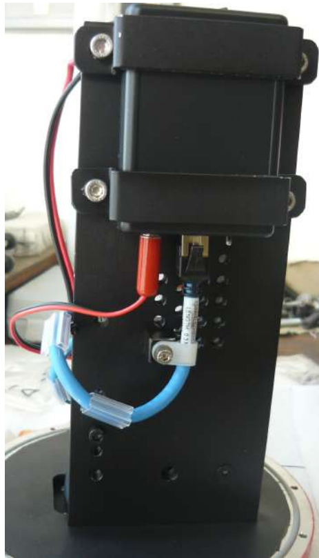
Figure 18. The SQM anchoring on the main mechanical frame.
