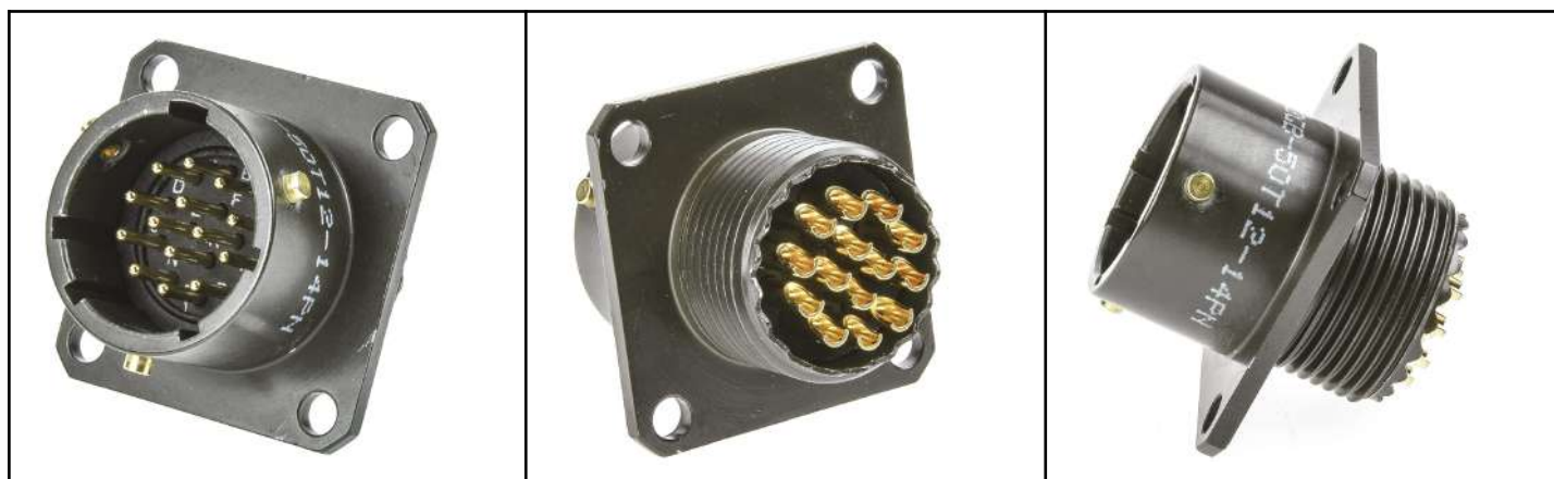
Figure 10. Amphenol Limited, 62GB 14 Way Flange Mount MIL Spec Circular Connector Receptacle, Pin Contacts, Shell Size 12, Bayonet Connector
