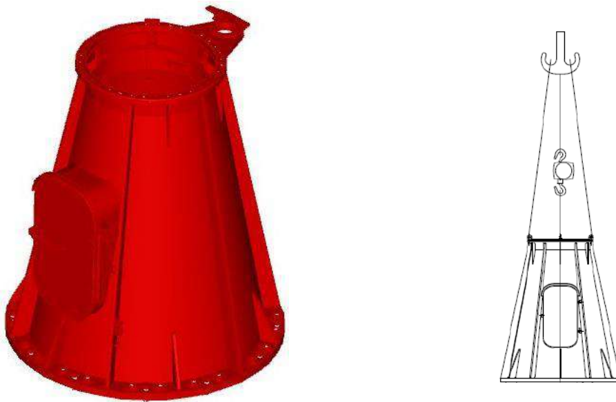
Figure 2 Base structure characteristics and lifting method
