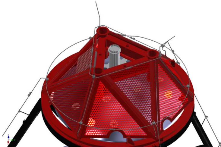
Figure 4-5: The PMC installed on top the M2 support Structure (courtesy of EIE Group SRL)
