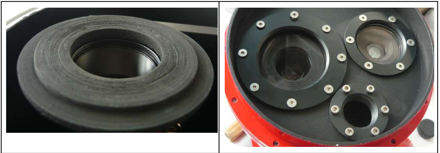
Figure 18. The PMC optical seal (left) and the Optical windows with the optical seals and devices below (right).
