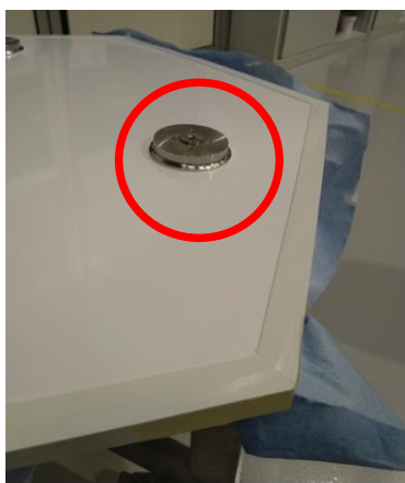
Figure 6 – Example of the “0” angle identification symbol etched on a pad.
