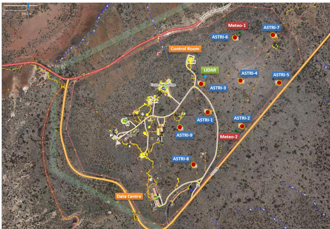
Figure 3-2 - The ASTRI Mini Array Layout at Teide Observatory. The big red dots indicate the positions of the ASTRI telescopes (ASTRI-1 to ASTRI-9).
