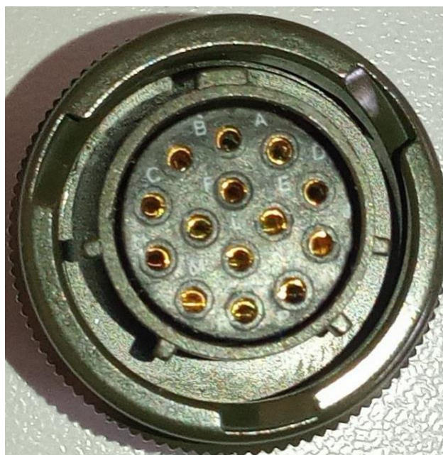
Figure 6. Amphenol Limited, 62GB 14 Way Cable Mount MIL Spec Circular Connector Plug, Socket Contacts, Shell Size 12, Bayonet corresponding to the male connector mounted on the PMC/SQM assembly plate.
