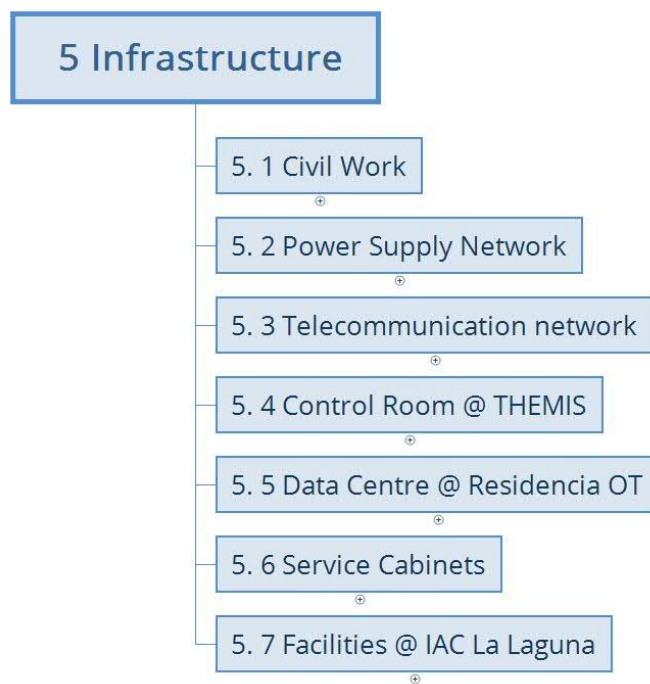
Figure 2. Product Breakdown Structure of the ASTRI Mini-Array on-site infrastructure.
