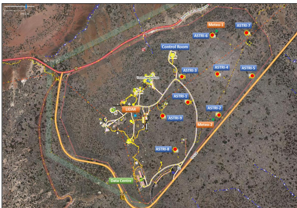
Figure 3: ASTRI Mini-Array general Layout The figure shows the final positions for the 9 telescopes, the roads to access each of them, the position of the two meteorological towers, the current position of the LIDAR, and that of the local control room (@THEMIS) and of the data centre (@Residencia). (Image obtained with Open Street Map editor)
