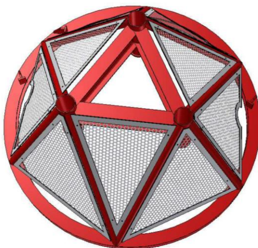
Figure 26. Top view of the M2 Support Structure (courtesy of EIE)
