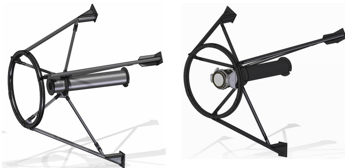
Figure 24. Left: the OSS Mast. Right: the mast with the Cherenkov Camera mounted (courtesy of EIE).
