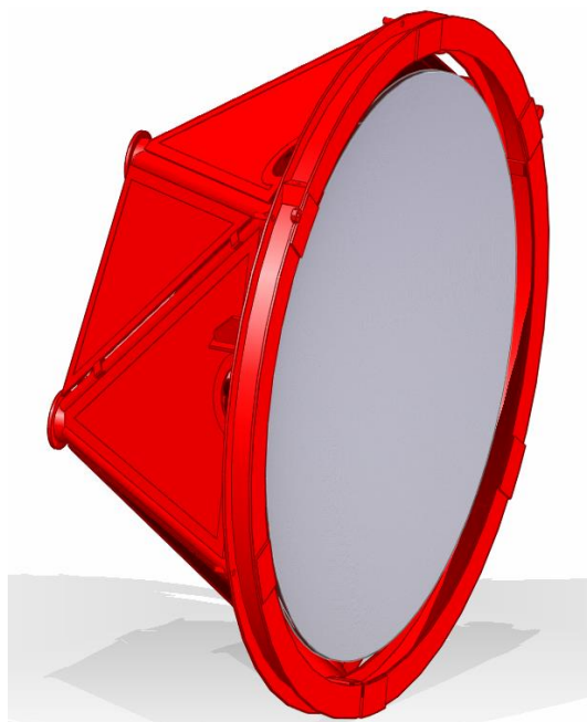
Figure 25. The M2 Support Structure (courtesy of EIE)
