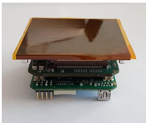
Figure 35. Camera Photo Detection Module. From top to bottom the SiPM board, the ASIC board and the FPGA board
