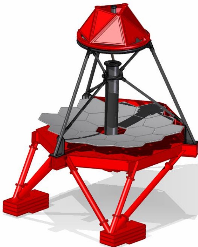
Figure 19. The Elevation Structure of the ASTRI Telescope (courtesy of EIE)
