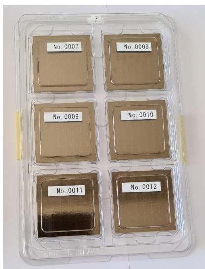
Figure 34. SiPM detectors' matrices.
