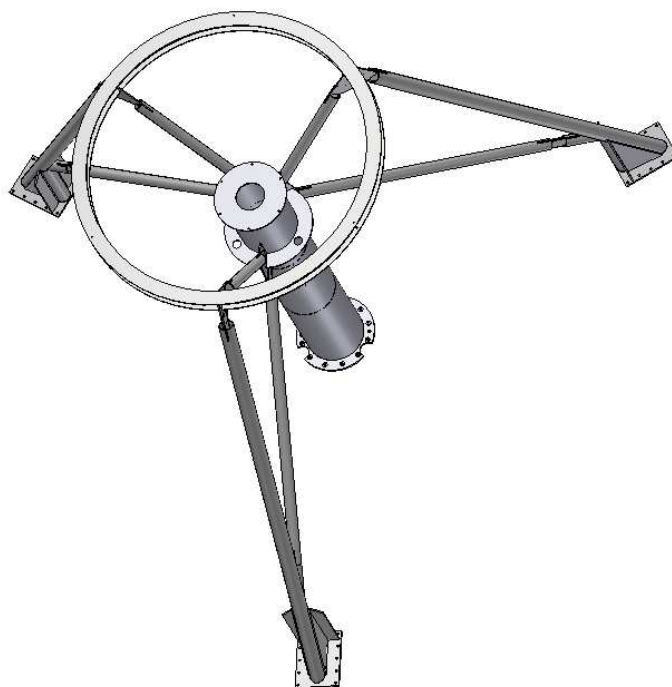
Figure 3-13 OSS Upper structure with mast and central tube
