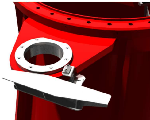
Figure 4-14 Azimuth stow pin witness details
