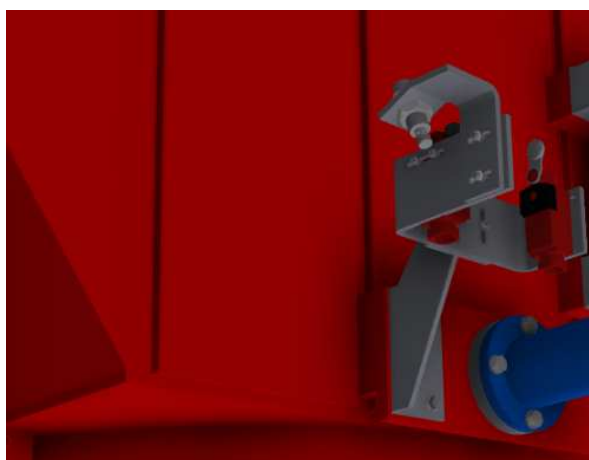
Figure 4-10 Elevation switches details
