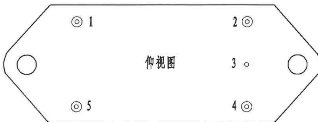
Figure 11. HFMH/ (20-50) -461-75 EMI Filter Outlet Arrangement
