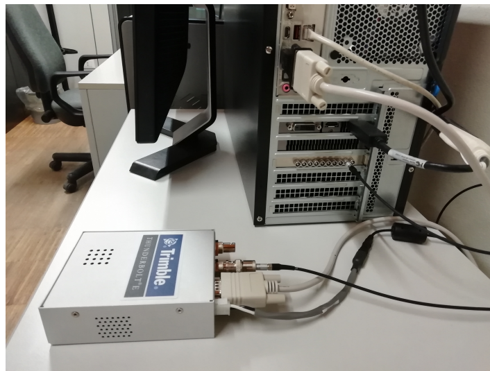
Figure 11. Top : Schematic representation of the components and internal connections of the BEE of ASTRI SI3. Bottom : Prototype version of the BEE mounted in the laboratory, tested with a PPS input signal from a GPS receiver.
