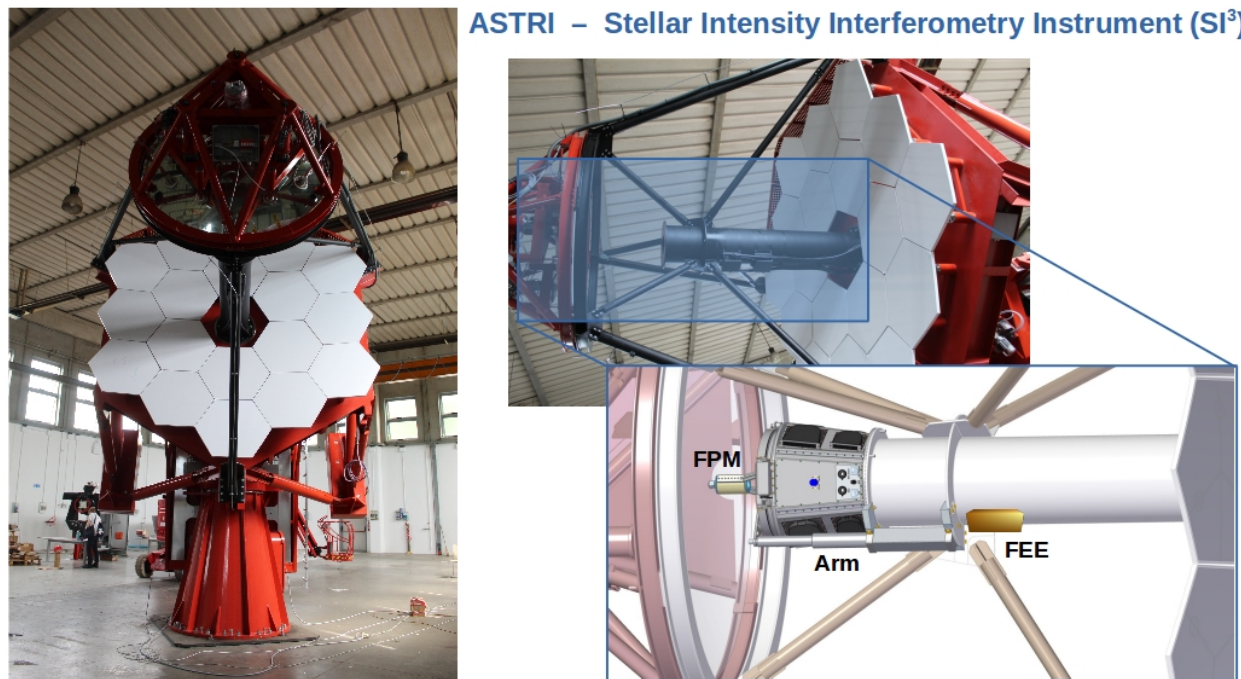
Figure 7. ASTRI telescope during factory assembly ( left ) and schematic view of ASTRI SI 3 ( right ), with the Focal Plane Module (FPM) deployed in front of the Cherenkov camera by the moveable positioning Arm and the box containing the Front End Electronics (FEE). The Back End Electronics (BEE) is located in the telescope cabinet and is not shown.
