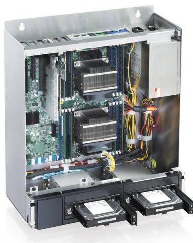
Figure 31 - IPC BECKHOFF C6670-0010. External (top panel) and internal (bottom panel) view.
