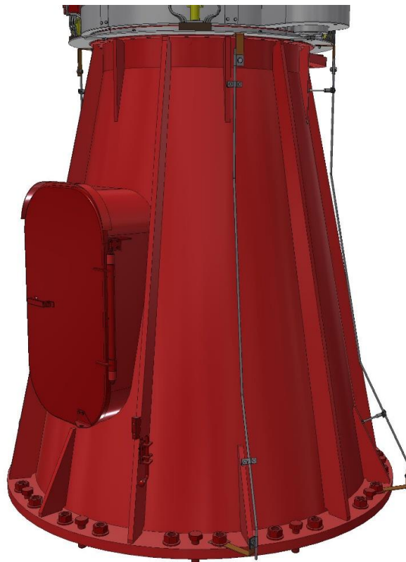
Figure 7-13: Base down conductors
