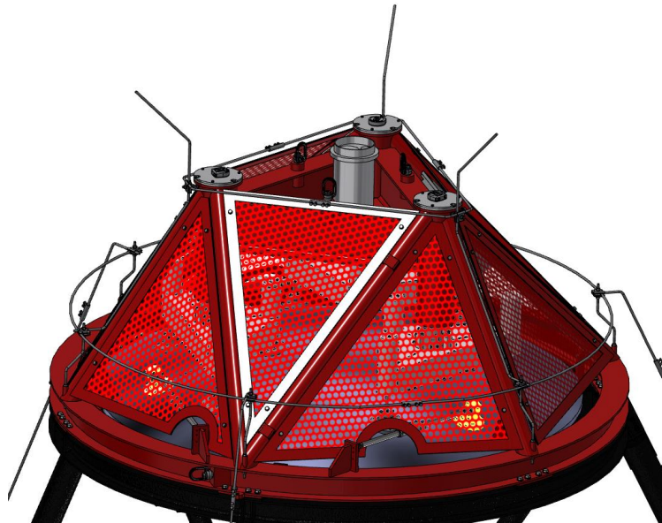
Figure 7-6: M2 Support structure air-termination rods
