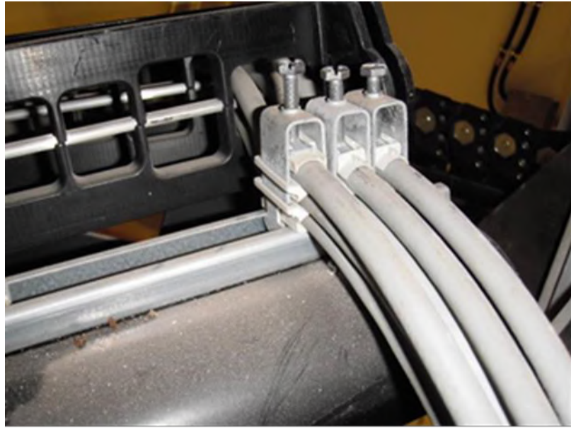
Figure 6-7: Applicative example of a clamp clips system
