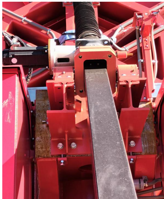
Figure 5-12: The ASTRI Mini-Array Telescope Elevation mechanism.
