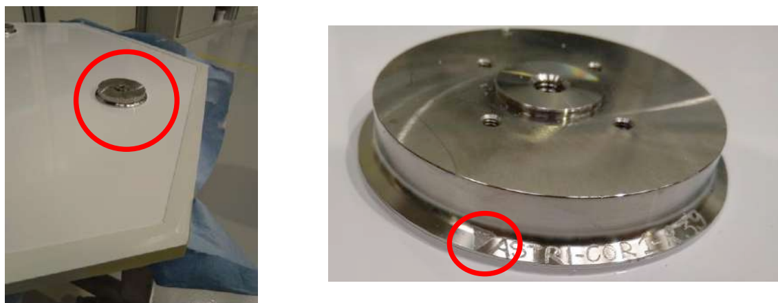
Figure 6 – Example of the “0” angle identification symbol etched on a pad.
