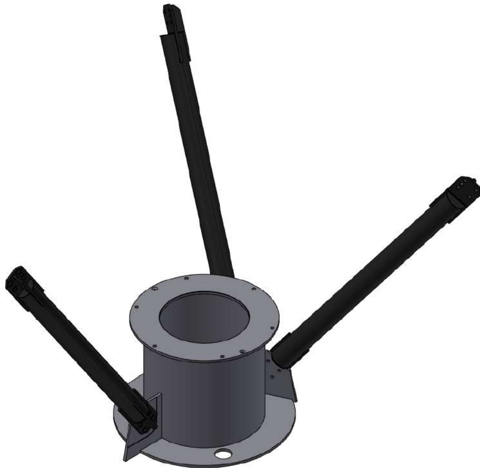
Figure 12: Camera Upper Support Structure, showing the interface flange where the Camera is connected.
