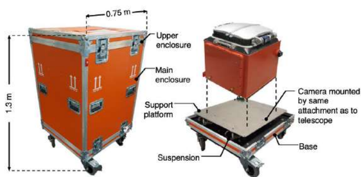
Figure 24: The custom wheeled transport container used for CHEC-S.
