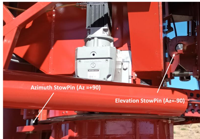
Figure 4-5 The stow-pins realized for the ASTRI Mini-Array telescopes
