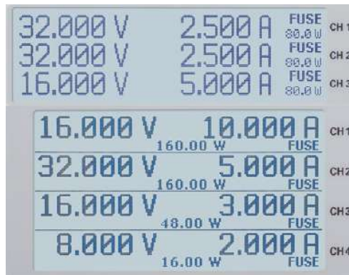
Fig. 4.7: R&S®HMP2030/ R&S®HMP4040 Fuse appearance in the display
