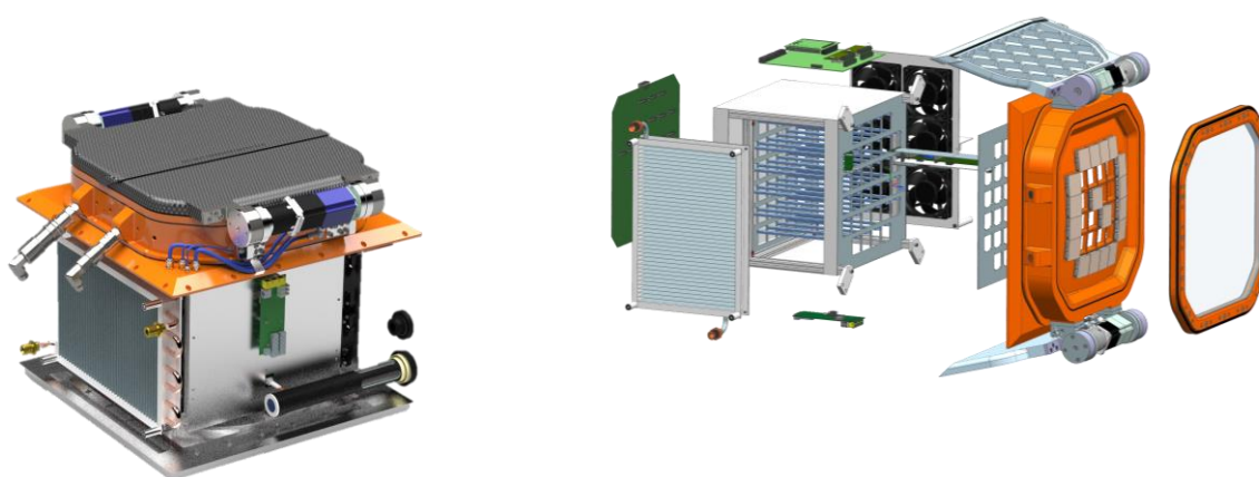
Figure 11-2 Left side: overall 3D CAD view of the Camera Unit (excluding enclosure); right side: exploded view of the unit showing some of the main components.
