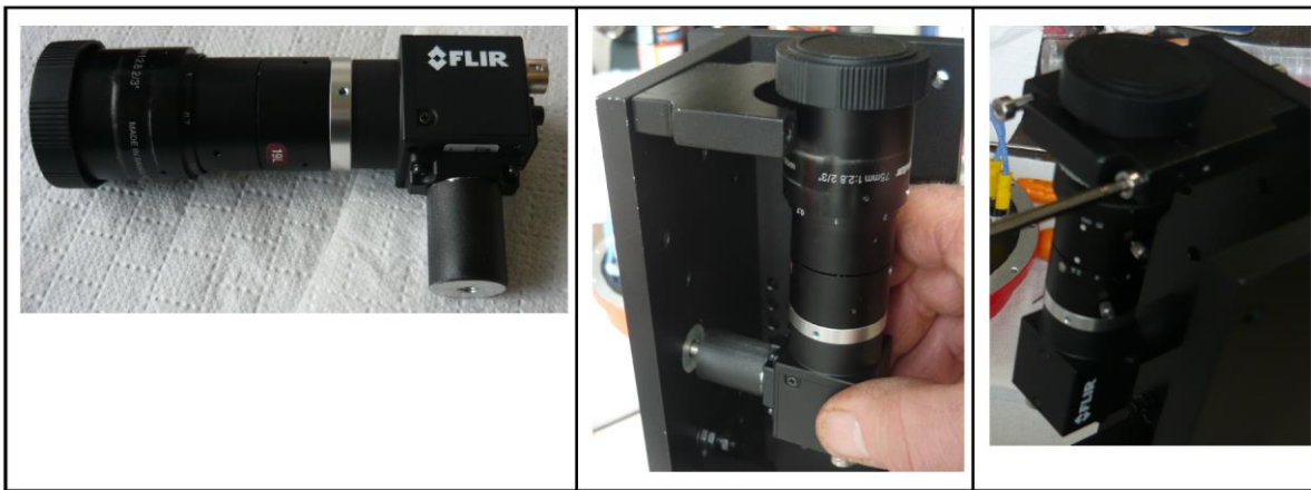
Figure 4-6: A picture of the PMC Camera and Lens assembled together with the metal cylinder used to anchor the camera to the main mechanical frame (left). The PMC/Lens while being mounted on the internal mechanical frame (centre and right).
